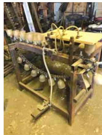
Homemade machine is operated by a foot pedal and uses air pressure and round-bottom cups to blow away garlic peels.
