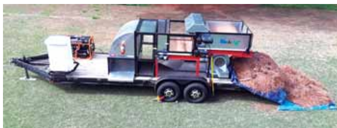
The Pine Bine uses conveyors and a fan to remove cones and sticks from pine straw, leaving only perfectly clean straw to be baled.
