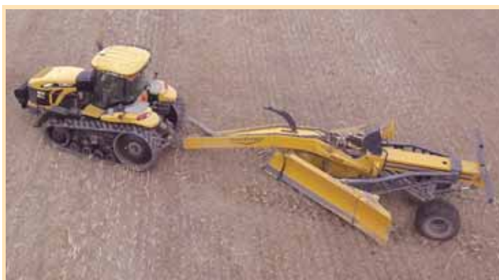
Terraformer 8650 comes with a telescoping frame and adjustable wing tips, allowing operator to form infinite "V" configurations.
