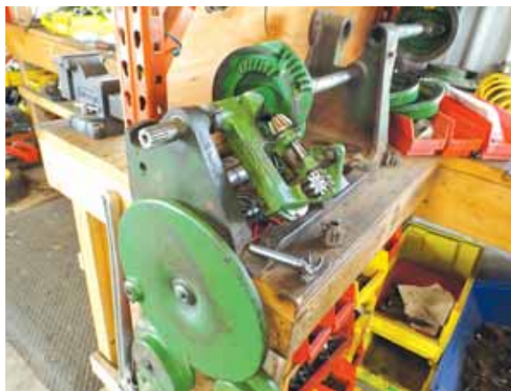
Finger Lakes Equipment rebuilds small square balers, often totally rebuilding the knotters or even the entire machine.
