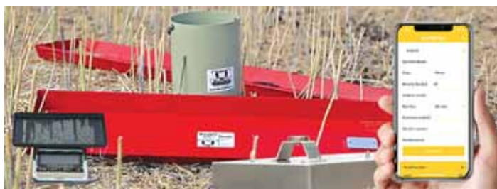
Drop pan attaches magnetically under combine and is dropped remotely while harvesting to collect a sample of chaff and straw. Sample is cleaned in an air separator and the remaining grain weighed on a scale. A downloadable app shows bu. per acre grain loss.
