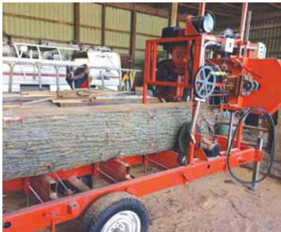
Dave Sager mounted a remote-controlled electric drive system on his bandsaw-type sawmill to make it run smoother and easier.
