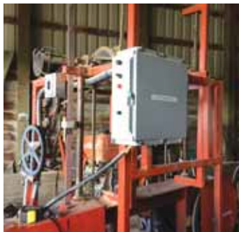
A 1/2 hp., 12-volt electric motor, geared down by a double sprocket drive, mounts on a saw head frame. A second electric motor raises and lowers saw head.
