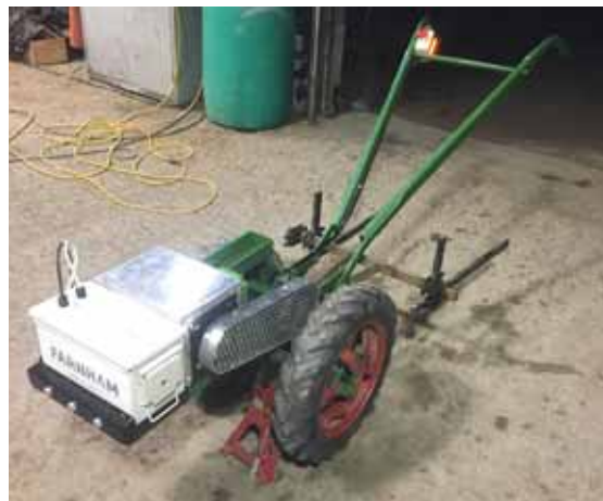
Two-wheeled, walk-behind tractor is operated by an electric motor from an old battery-powered floor scrubber.
