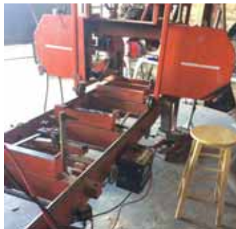
A 1/2 hp., 12-volt electric motor, geared down by a double sprocket drive, mounts on a saw head frame. A second electric motor raises and lowers saw head.
