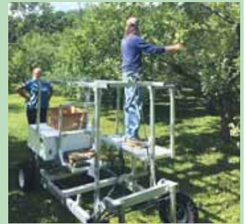
Adjustable steering wheel and throttle allows operator to stand and pick apples with the steering wheel right next to him.
