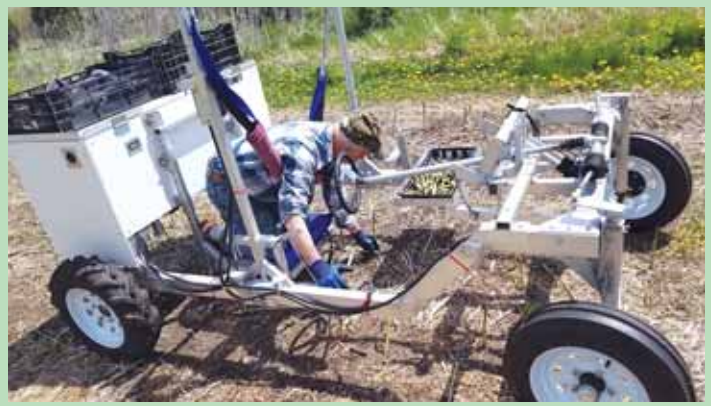
Cart is designed so operator can kneel forward on a chest support, and also sit or stand. Photo shows cart set up to plant asparagus.
