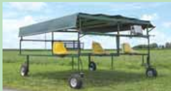
Battery-powered portable canopy provides shade, seats, fans and racks for cold water. It was designed for tobacco field work to go in 36-in. rows.
