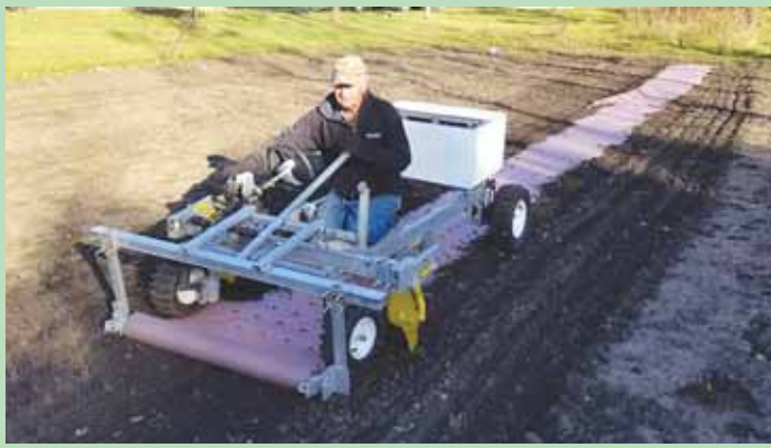
Dean Maschoff uses his modified golf cart to do a variety of jobs that make gardening work easier. Here he's laying down paper mulch.
