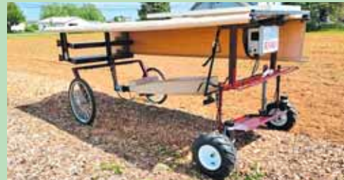
Solar-powered RoHand II crop cart has a canvas top with roll-down sides that protect the operator from sun or rain.
