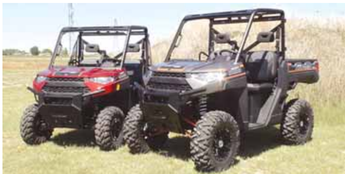
Photo shows the difference between a 2020 stock Polaris Ranger (left) and a Ranger equipped with a Marshall Motoart 2 1/2-in. lift kit.
