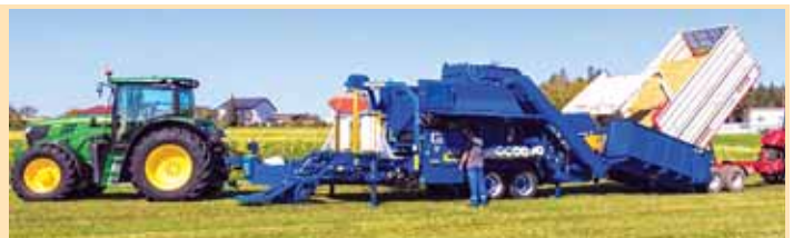
Goeweil baler-wrapper compresses material more tightly than a conventional baler-wrapper. It can compress and wrap almost any material, including corn silage.
