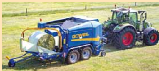
The F125 Kombi baler automatically bales and wraps airtight bales in one operation, resulting in unsurpassed feed quality, says the company.
