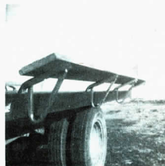
Special strut on bracket prevents distortion of stake holes.
