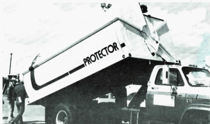
Two small cylinders mounted across the front of the box open and shut the lids.
