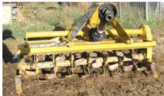
Siegrist added tines - cut down from old field cultivator teeth - to the skids on his compact tractor-mounted rototiller to let it dig deeper.
