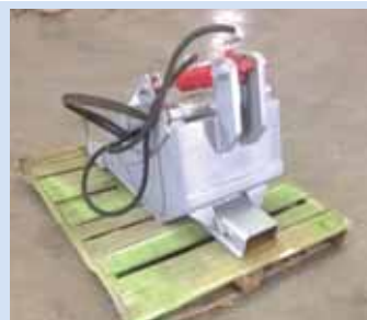
Receiver tube on "Power Bar" accepts a wide variety of attachments, including the forage fork shown at right. "It eliminates need for a separate quick-tach plate for each tool," says inventor Howard Popp.
