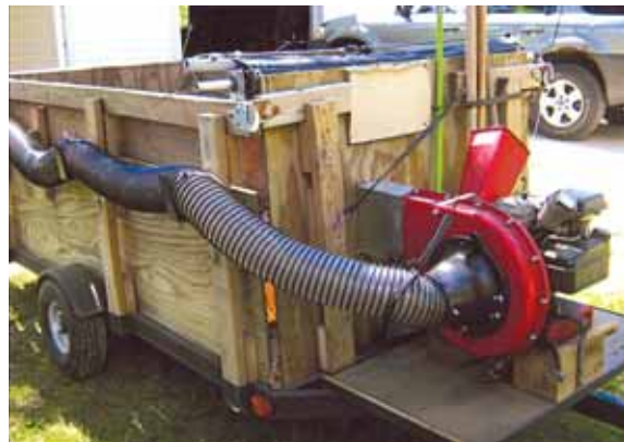
Converted wood chipper shreds branches as well as leaves and blows the material into home-built trailer.
