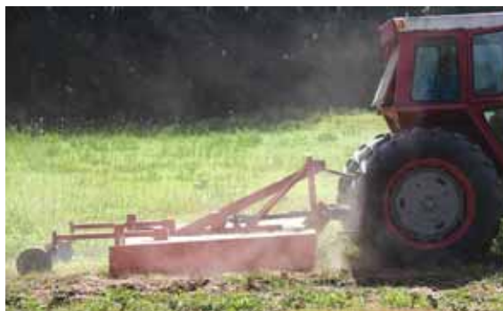
Home-built, 7-ft. bush hog rides on caster wheels on back and has a 1-ft. deep deck with an old-style, squared-off look.
