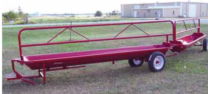
Towable 14-ft. feed bunks can be hooked together to tow behind a tractor or pickup. Bunks are steerable so each one follows in the track of the one ahead of it.
