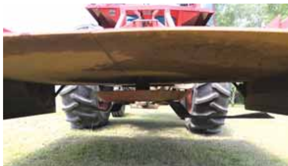
A stump jumper is attached to bottom of mower's gearbox, with the blades bolted to it.
