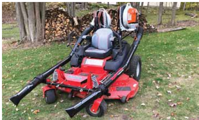
Redesigned leaf blowing system features adjustable pvc pipe mounts, rotating nozzles, and a simpler leaf blower mounting system.
