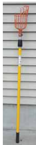
Johnson replaced the 5-ft. wooden handle on his fruit picking tool with a paint roller extension pole, extending the length to 16 ft.
