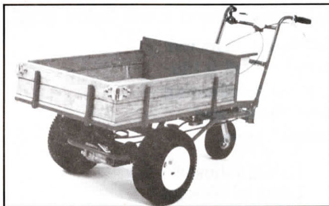
Cart has two up-front drive wheels powered by a belt-driven transaxle.
