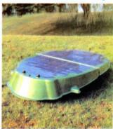
The mower is fitted with extra-sharp tungsten blades that turn so slowly they pose no threat of injury to people but turn just fast enough to cut grass. The mower moves ahead at a maximum speed of 1 1/2 ft. per second and can work slopes as steep as 30°.
