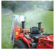
"Coverage is better than with an air blast sprayer that applies spray to the lower leaves, but requires a handgun to reach the upper branches. The Munckhof creates a smooth, laminar column of air the length of the tower. Droplets are formed to the correct size and pattern before entering the air stream. The Munckhof can be adjusted to the height of the trees and turns the leaves to the side to spray both sides.
