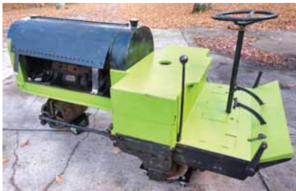
Ricci owns this rare 1917 J Coldwell Model J lawn mower that is missing its front cutting reel.
