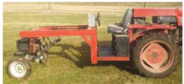
One-of-a-kind cultivating tractor was built to run between the 48-in. rows in Davis's garden.
