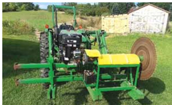
Frame-mounted buzz saw blade quick-taches to the loader arms on Kring's 4-WD tractor.
