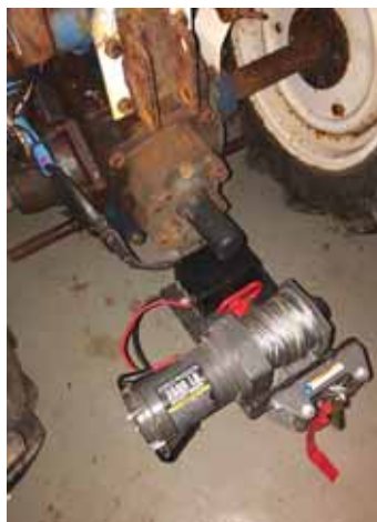
Remote-operated electric winch is bolted to a homemade bracket that slides onto tractor's drawbar.
