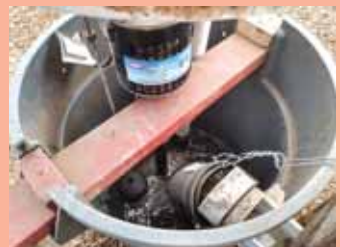
Submersible pump in trash can (above) sends water back to stock tank. Chickens drink out of a 4-in. pvc pipe with the top sliced off to form a trough.
