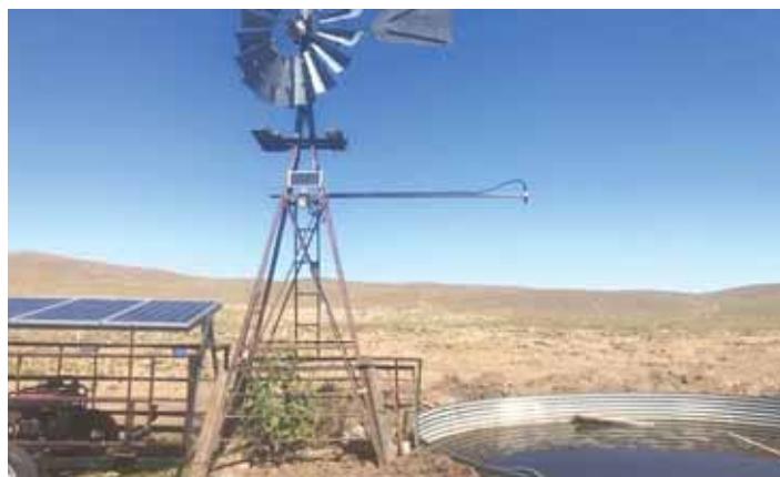
Solar-powered Tank Toad uses submersible pressure sensors, or sonar sensors, to measure the water level in remote stock tanks.
