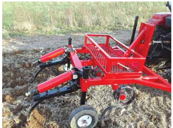
Chisel CR deep tillage tool has 2 rear shanks spaced 3 ft. apart, which dig the soil up to 14 in. deep.
