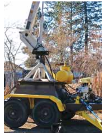
Boom is bolted to a 2 1/2-ft. tall, trapezoid-shaped frame equipped with a 5-ft. square base.
