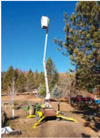
Malcolm mounted the boom from a bucket truck on a trailer. "Works great to reach out over a thick patch of berries," he says.
