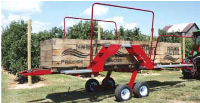
Flow Thru Harvester is designed to pick up crates filled by ground-level pickers. As it moves down the row, crates are gradually carried up an incline.
