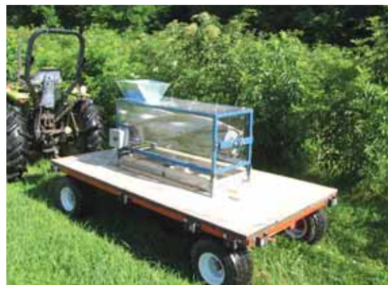
"Destemmer" uses a section of flighting inside a hardware cloth drum to destem clumps of elderberries, which are fed into a hopper on front.
