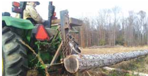
Jack Agnew says his home-built, 3-pt. log lifter works great to move logs to his sawmill.
