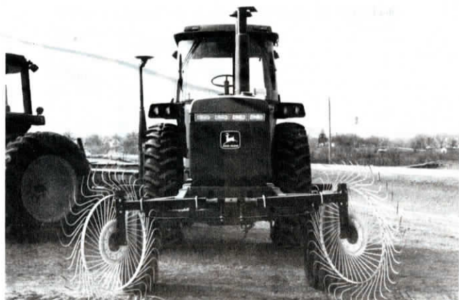
"Hay Guides" consist of a pair of 55-in. dia. rake wheels mounted on a frame that clamps to the front of your tractor.
