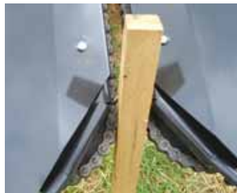
Two-wheeled Stake Puller uses a pair of hydraulic-driven roller chains (below) to pull stakes out of the ground and deposit them on a rack.
