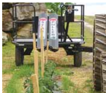
Two-wheeled Stake Puller uses a pair of hydraulic-driven roller chains (below) to pull stakes out of the ground and deposit them on a rack.
