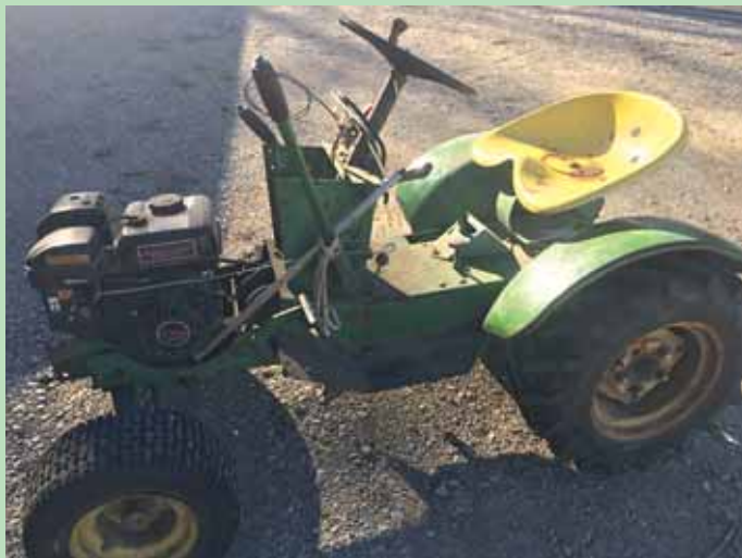
Tschetter says the Harbor Freight Predator 6.5-liter engine he installed in his Deere 110 garden tractor "works great, and I saved a lot of money."
