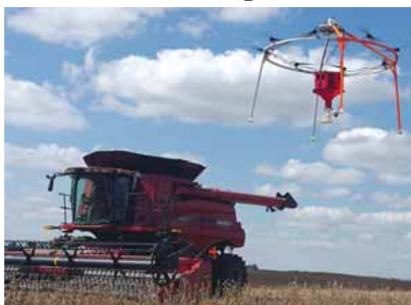
AeroSeeder drone is 65 in. in diameter. Controlled by GPS positioning, it can seed up to 100 acres in 8 hrs.
