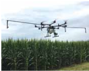
Drones can be equipped with a liquid tank and spray boom, or a dry spreader.
