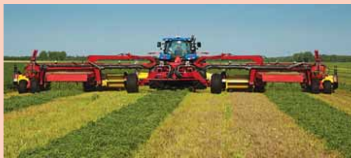
Triple Cutter Toolbar can carry 16 to 18-ft. New Holland HS sickle heads, or 16-ft. MacDon R85 disc heads. One head is mounted on front of tractor, producing a combined cutting width of 40 to 54 ft.
