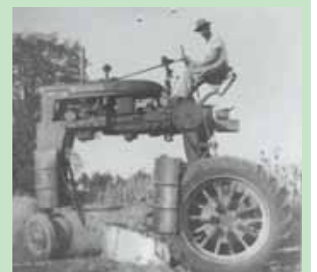
Mounted-on-stilts Farmall was used in the 1950's to plant wheat between rows of standing corn before harvest.
