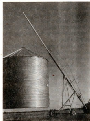
Bin Crane raises to 45 ft. and lowers to 14 ft. for transport.
