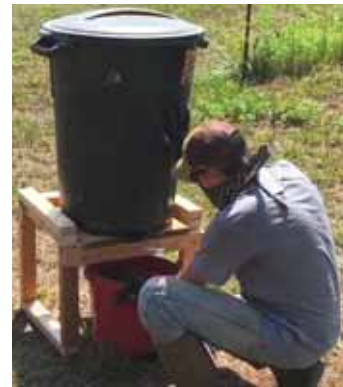
Barrel fitted with slide valve sets on a wooden stand, high enough to place a 5-gal. pail underneath to catch the grain.
