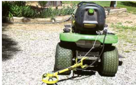
String trimmer on back of mower is free to move forward or backward, out of the way of trees and rocks.
