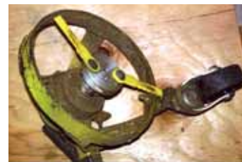
Trimmer head is equipped with a pair of serrated plastic blades, which bolt onto a hub attached to 12-volt motor.
