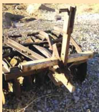
Homemade hitch lets Waldner use small tillage implements designed for a 25 hp. Farmall, with his bigger Deere tractor equipped with a 3-pt. hitch.
