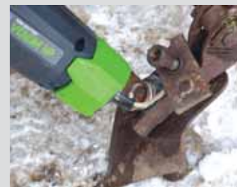
Insulated electrode on tool focuses electromagnetic energy only on the parts you're working on.
