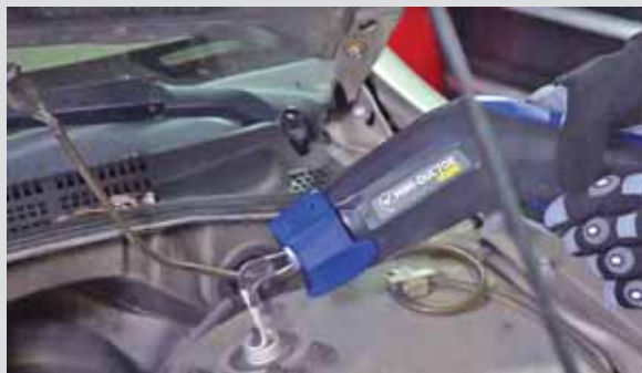
Mini-Ductor Venom tool uses flame-free heat to loosen rusted bolts and other parts.
