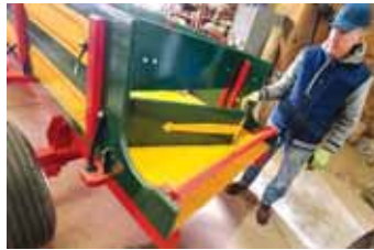
Two-piece hinged endgate on back of wagon is used to shovel corn out by hand.
