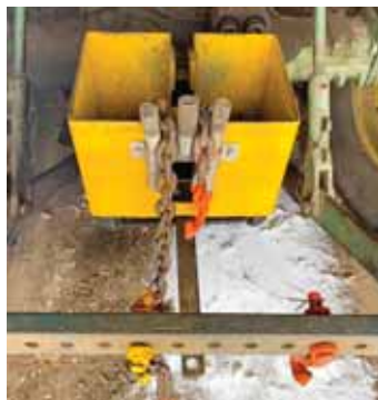
Springs on chain holder allow chain to feed out safely if it ever unhooks from grab hook on crossbar.
