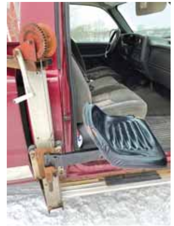
Boat winch raises and lowers carriage-mounted seat, which also swings out.
