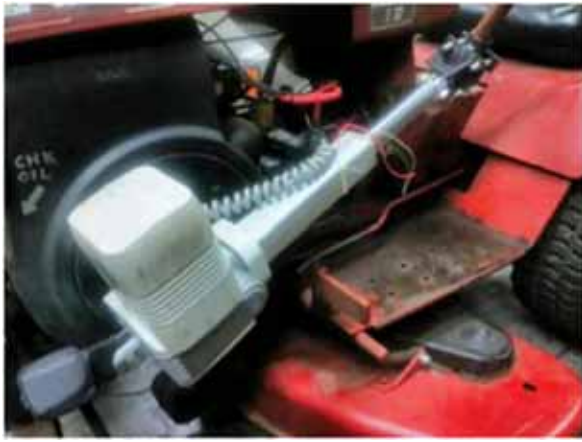
Reining added electric lift to his Wheel Horse by installing a 12-volt electric screw jack between the tractor's frame and existing lift handle.
