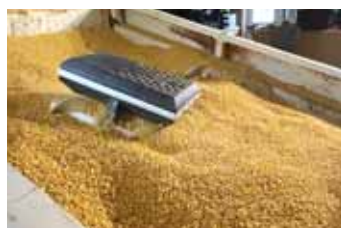
Remote-controlled robot is equipped with two 6-in. drive augers, allowing it to drive across grain and level it or tear up the crust.
