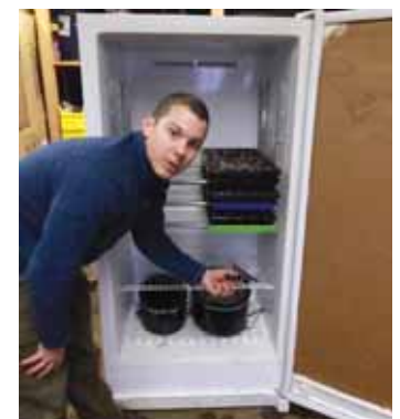
Water-filled Crockpots release heat and humidity into refrigerator chamber, helping seeds to germinate.
