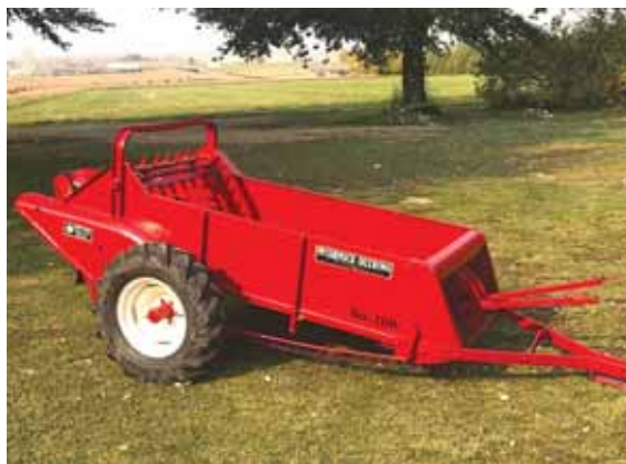
Lar Voss rebuilt this 70-year-old McCormick Deering 100 ground-driven manure spreader, even building a new cam to replace the broken one on the spreader.
