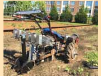
Walk-behind transplanter has a powered no-till coulters, double disc openers, and closing wheels.
