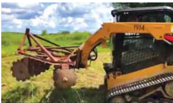
Rogers adapted an old 3-pt. mounted, 10-ft. disk to use on his Terex track loader by welding a quick-tach plate on back of disk.
