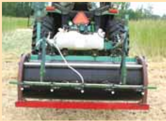
Specially designed herbicide applicator can be added to any roller.
