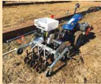
Three-row drill for walk-behind tractors carries a 1/2-bu. seed hopper.
