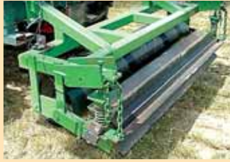
Two-stage roller crimper has a smooth roller followed by a straight bar crimping roller.
