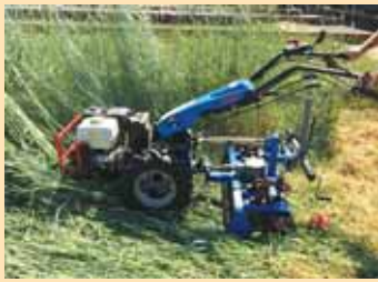
Pto-driven walk-behind roller/crimper works great for smaller operations.
