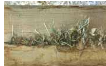
Concrete nails extend 2 in. below dethatcher's front board to stir up soil and bury grass seeds.
