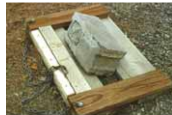
Concrete nails extend 2 in. below dethatcher's front board to stir up soil and bury grass seeds.
