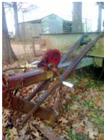
Tilt trailer is raised or lowered using a hand-cranked, winch-operated hoist and jack attached to trailer tongue.
