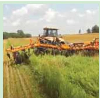
Elixir models have a 40-degree range of motion for uneven terrain.
