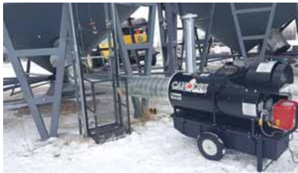
Portable dryer is powered by 2 indirect-fired diesel fuel burners, which blow heated air into the grain through a 12-in. rigid spiral pipe.
