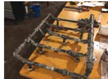
Water enters and exits the firewood-holding grate through separate outlets at the front. Heated water is pumped down through PEX pipe to a 12-in. sq. “water to air” heat exchanger in basement (below).
