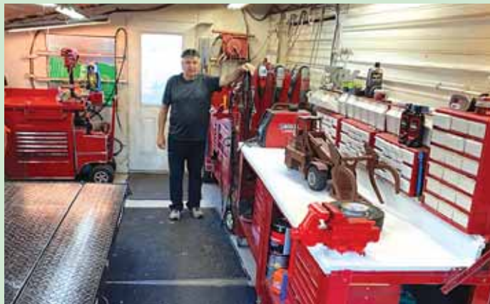
Steel tables have proven to be useful for creating work spaces, and Campbell has several to which he attached kitchen countertops.
