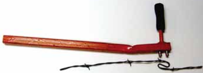
LeRoy Momper made this simple tool to keep his wire fences tight. Each twist takes up about 1 1/2 in. of slack.
