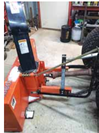
Reverser lets Olds mount a front-mount snowblower on back of his Deere tractor.
