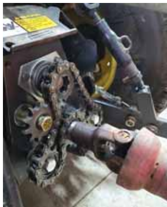
Pto reverser uses tractor's factory pto shaft to chain-drive a second pto mounted below.
