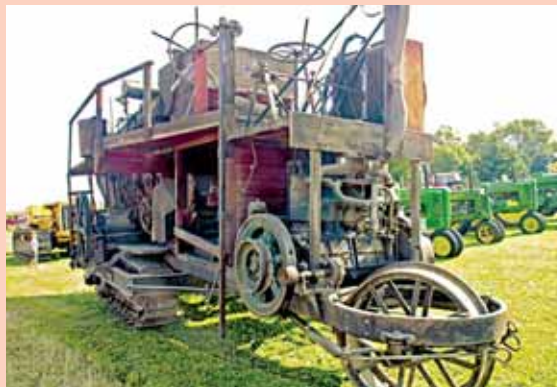
It took a crew of 5 men to operate this rare 100-year-old Holt self-propelled, tracked combine, which is now owned by Josh Stephenson in California.
