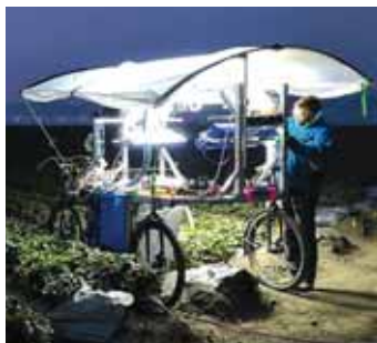
Researchers gather crop data from this robotic, wheel-mounted buggy that’s fitted with cameras and uses artificial intelligence.
