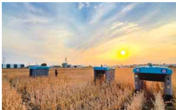
These 3 different types of robots are named Tom, Dick and Wilma. If Wilma identifies the plant as a weed, then Dick is dispatched to zap it.
