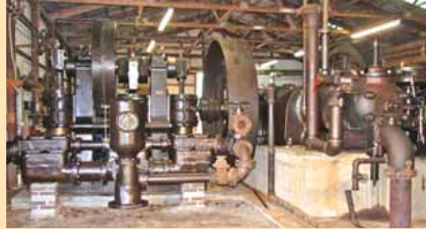
This rare 75 hp. Otto engine is one of only two surviving 1912 models.
