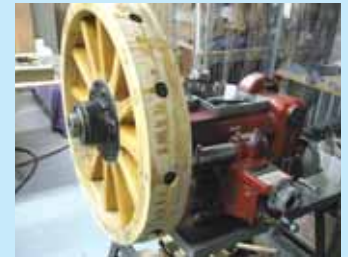
One of their toughest jobs was building new wooden wheel rims to replace those that were rotted and filled with holes.
