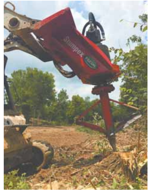
Skid loader-mounted Stumpex cutter bit uses weight and high torque while operating at a low 7 to 17 rpm’s. The slow speed reduces flying debris.
