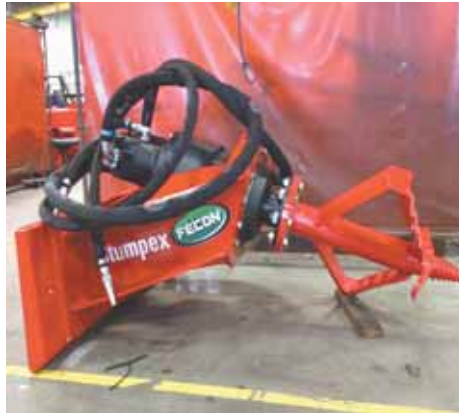
Skid loader-mounted Stumpex cutter bit uses weight and high torque while operating at a low 7 to 17 rpm’s. The slow speed reduces flying debris.
