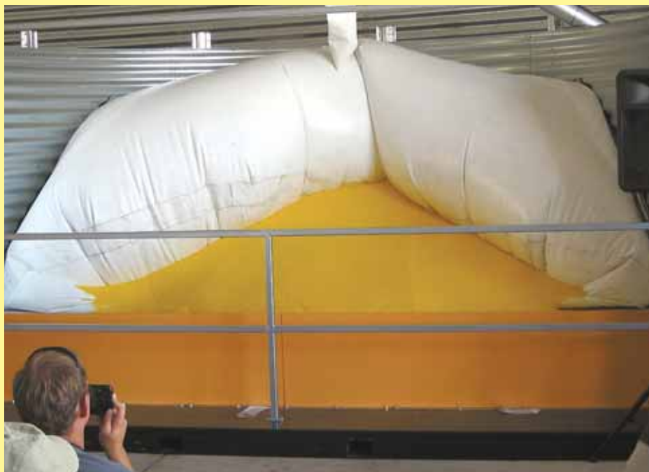
Photo shows one half of floor liner inflated, channeling grain towards the unload auger.
