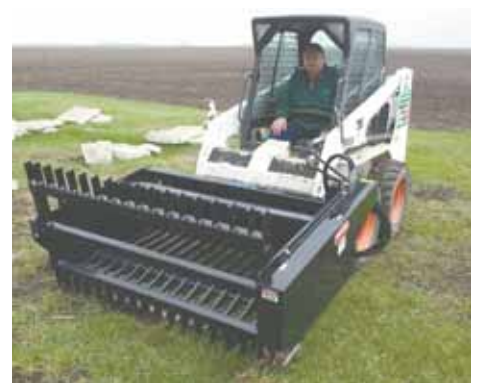
Rock picker's front-mounted reel flips rocks into bucket. "It gets both big and small rocks," says inventor Lester Pritchard.
