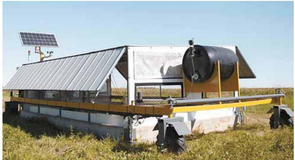
Solar-powered robotic chicken coop moves automatically and carries a week's worth of feed and water. It can be controlled from a smartphone. "Because it's fully automated, I spend only 5 to 10 min. a day checking on my chickens," says Daniel Badiou.
