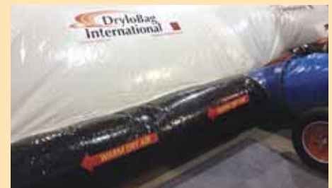
Side tubes on latest bags are black, which raises the temperature of air blown into grain.
