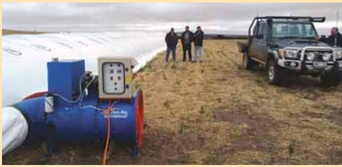
Grain is loaded into bag with standard bagging machine. Dryer hooks to plastic tube on side of bag, sending warm air through grain and out tube on other side of bag.
