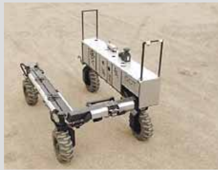
Powered "platform" has 4 hydrostatically-driven wheels.
