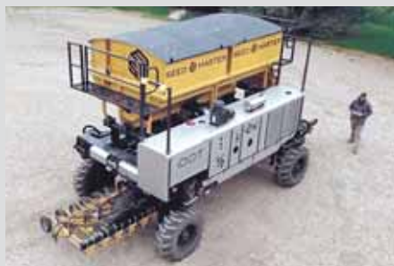
Once docking is complete, the computerized platform can be controlled by a remote operator or it can run itself, controlled by GPS.
