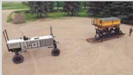
Grain drill (right) was designed to fit platform, which drives under and lifts it into place before heading to the field.
