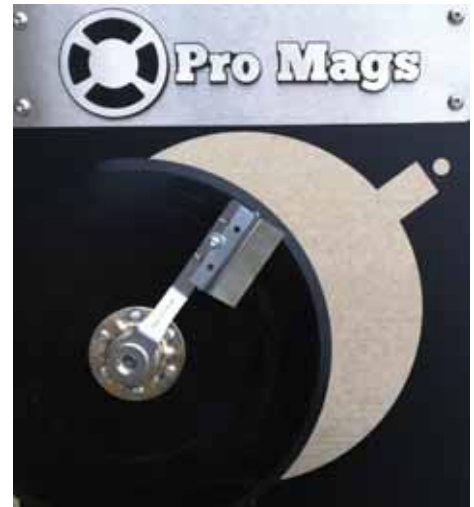
Universal scraper bolts onto the axle of any planter’s opening disc.
