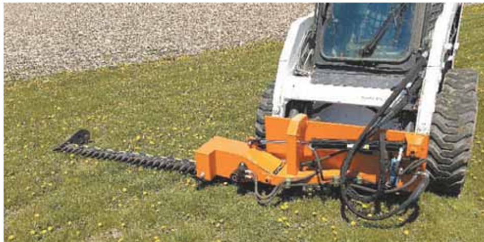
"It's handy for doing a variety of farm work," says Andrew Lee, who converted a New Idea pto-powered, 7-ft. sicklebar mower to hydraulic-drive for use on his Bobcat skid loader.
