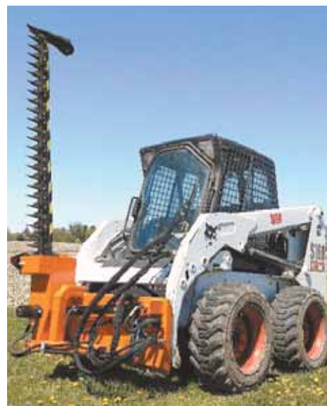
Mower folds up vertically for transport and downward for roadside clearing.
