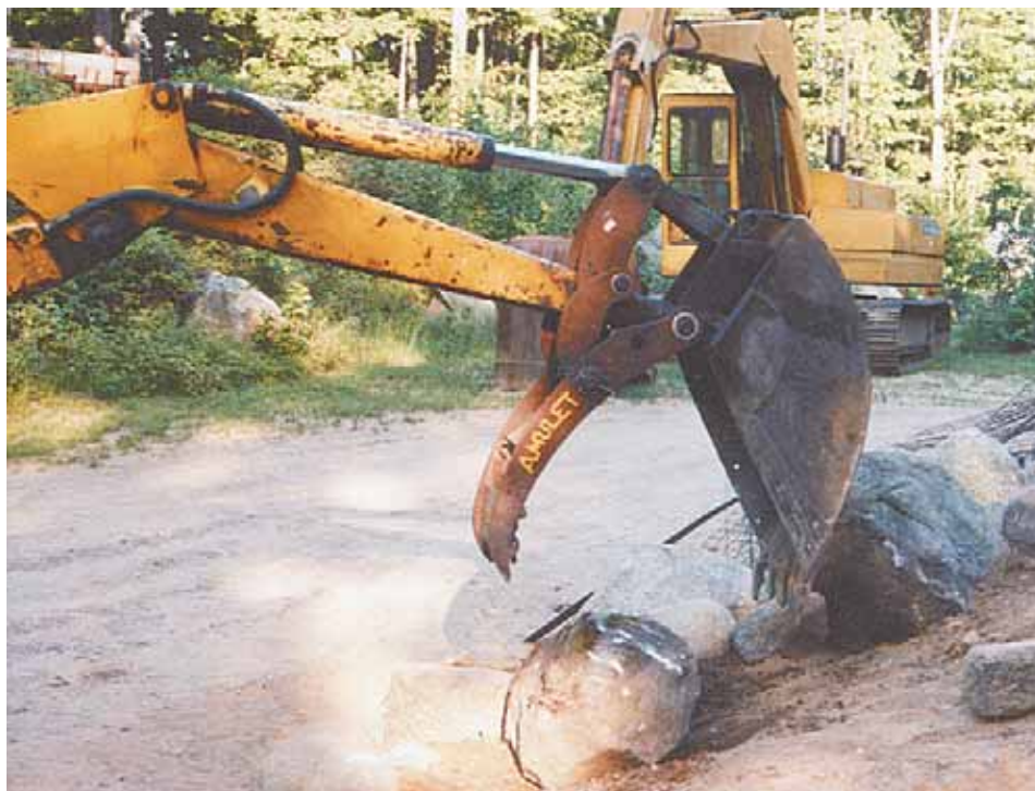
HoeClamp moves as bucket moves. Lund says it’s easier to use than a “hydraulic thumb”.
